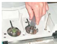
Use the smaller end to remove the septum nut.
