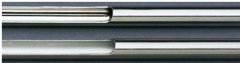
Top: electropolished finish, surface roughness average number: 5-10. Bottom: conventional finish, surface roughness average number: 23-27.
