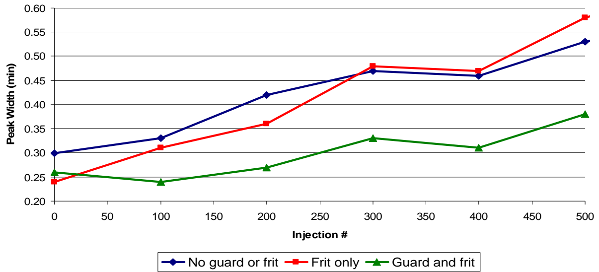
Figure 4: Amiodarone Peak Width Over Column Lifetime
