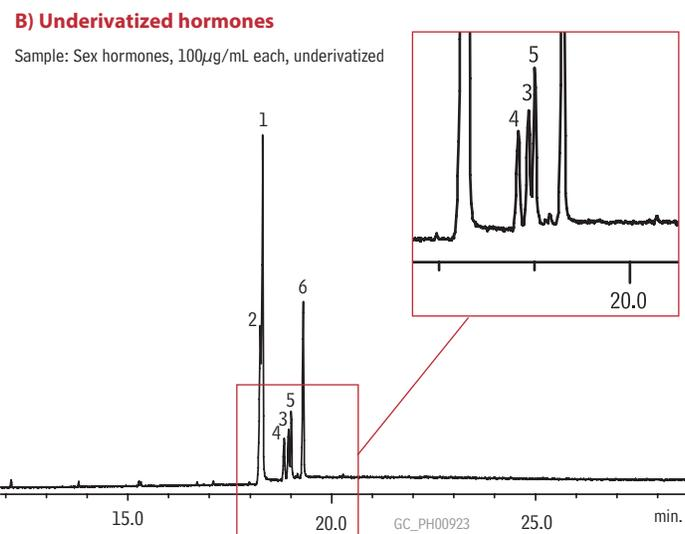
Column: Rxi®-1ms 30m, 0.25mm ID, 0.25µm (cat. # 13323)
