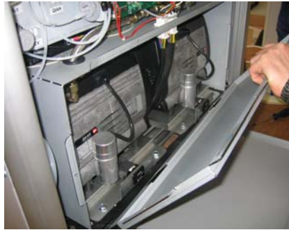
Fig. 9-10 – remove second cover
