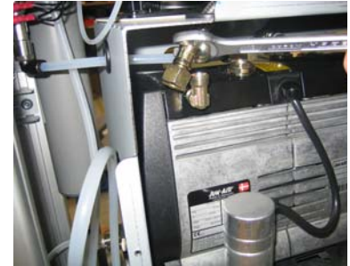
Fig. 9-11 undo bull nose connections
