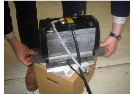
Fig. 9-17 – remove transit support blocks
