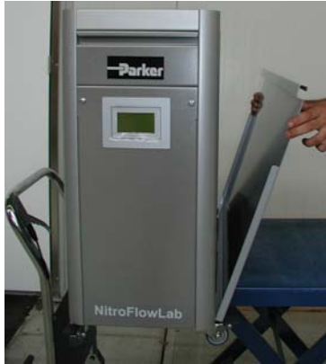
Fig. 9-9 – unscrew side panels
