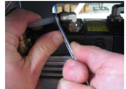
Fig. 9-14 – pull away pipe
