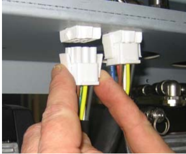
Fig. 9-15 – disconnect multi-pin plug
