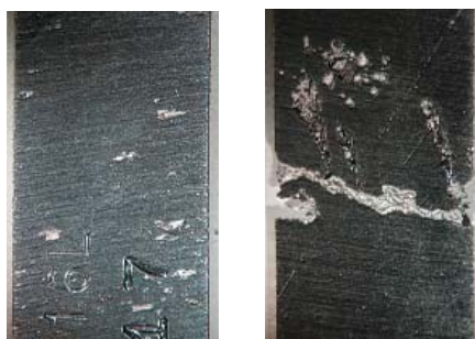
Figure 1 Silcosteel®-CR treated 316L stainless steel coupons show no crevice corrosion and only slight pitting corrosion; untreated coupons exhibit severe crevice corrosion.
