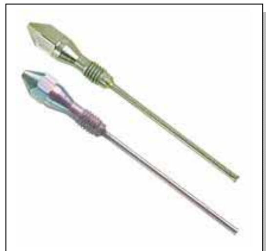
Fig.13 SS and Siltek deactivated flame tips for agilent FID
