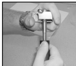
Figure 3: Resurface the sealing ring at the base of the injector.
