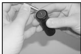
Figure 2: Place the sanding disk over the threaded post.
