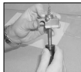
Figures 4 & 5: Clean injection port by moving the handle up and down several times inside the injector.
