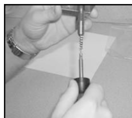
Figures 4 & 5: Clean injection port by moving the handle up and down several times inside the injector.
