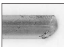
A bad column cut.
