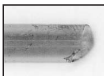
A bad column cut.
