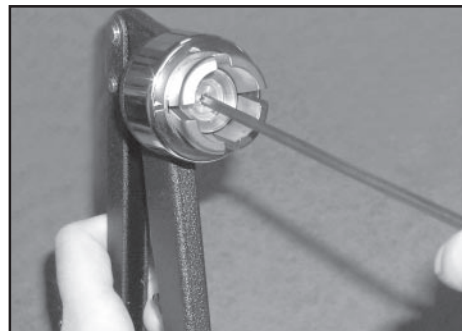
Figure 5—Coarse adjustment. Note allen wrench and coarse adjustment. Counterclockwise increases crimp. Clockwise loosens crimp.
