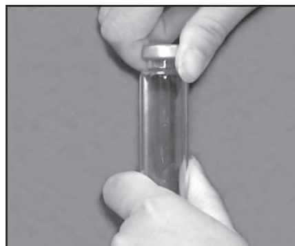
Figure 2—Under-crimped seal. Note that the seal may look properly crimped, but still can be rotated by hand around the vial.
