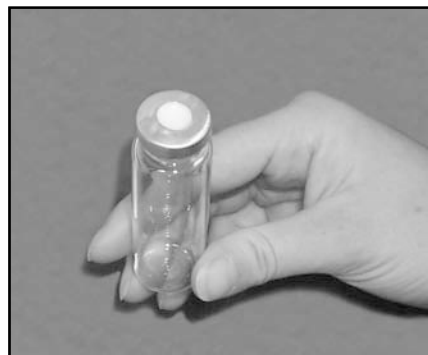
Figure 3—Over-crimped seal. Note how the seal is deformed around the sides and at the top. While a seal is obtained with this crimp, the deformed sides and top may interfere with the autosampler, headspace unit, or syringe. Poor system reliability may result from using over-crimped vials.
