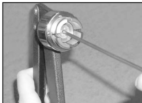
Figure 5—Coarse adjustment. Note allen wrench and coarse adjustment. Counterclockwise increases crimp. Clockwise loosens crimp.
