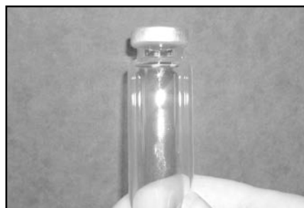
Figure 1—Good Crimp. Note that the crimped seal cannot be rotated around the vial.
