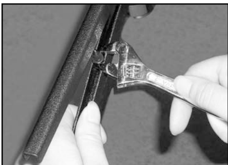
Figure 4—Fine adjustment. Note locking nut and adjustable height stop. Clockwise lowers height stop, increases crimp. Counterclockwise raises height stop, loosens crimp.
