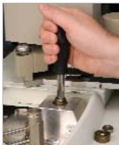
Turn counterclockwise to loosen liner cap.
