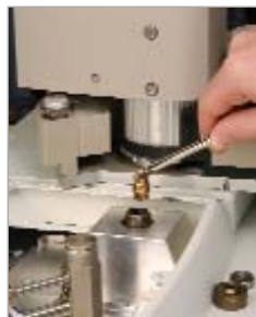
Use tweezers (cat. #20101) to remove liner cap.
