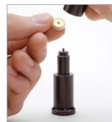
Pull the Assembly Tool apart and remove assembled Outlet Cap and Gold Seal.
