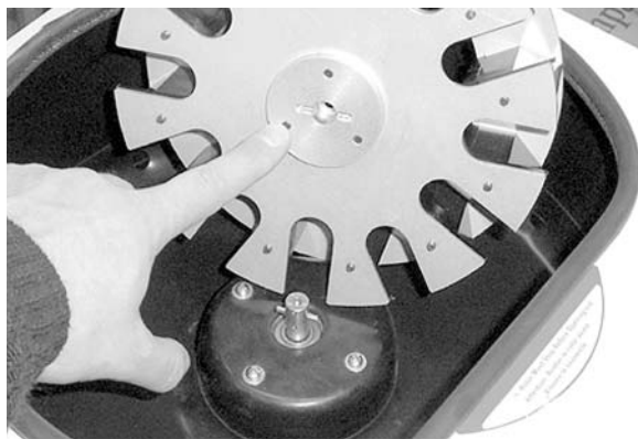
The slot in the bottom of the rotor must be aligned with the pin in the motor shaft!
