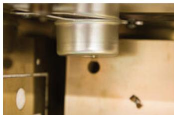
B) Extended reducing nut with insulating cup installed.
