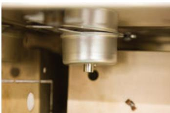
C) Column installed using extended capillary and reducing nuts.
