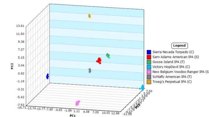
**Figure 5** PCA plot obtained with Mass Mountaineer<sup>TM</sup> from the MS profile data of sample sets of seven different Indian Pale Ale (IPA) beer samples.
