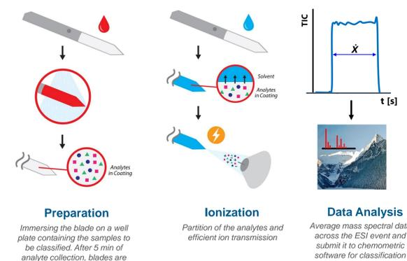
**Schematic 1** Representation of the sample preparation, ionization and data processing steps carried out using CBS technology for food safety applications.
