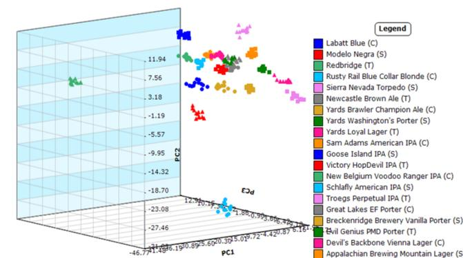
**Figure 4** PCA plot obtained with Mass Mountaineer<sup>TM</sup> from the MS profile data of sample sets of twenty different beer samples.
