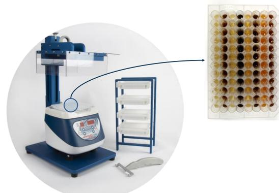
**Figure 2** Sample Handling Unit (SHU) used for simultaneous analyte collection with 96-CBS blades.
