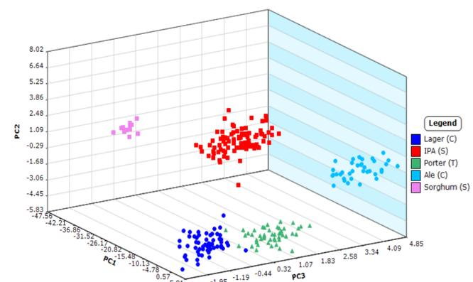
**Figure 3** PCA-DAPC plot obtained with Mass Mountaineer<sup>TM</sup> from the MS profile data of sample sets of five different beer classes.
