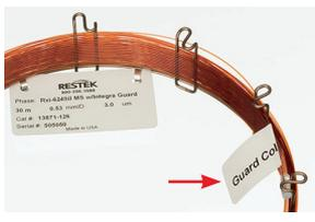
**Figure 3:** High-temperature string indicates where the Integra-Guard section ends and the analytical column begins.
