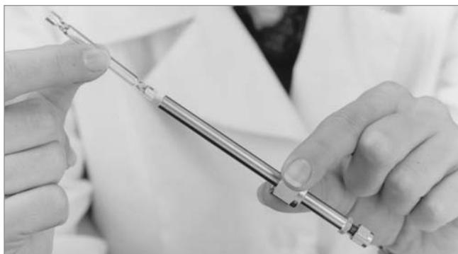
2. Connect the Uniliner® Inlet Liner Adaptor to the injection port, using the 1/4-inch stainless steel nut provided. Tighten the nut 1/4-turn past finger-tight.
