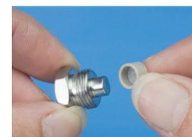
The cap frit can be easily replaced if it becomes contaminated/plugged.
