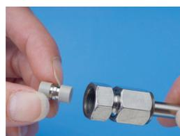
Remove the XF end fitting and install the guard cartridge in the end of the column.
