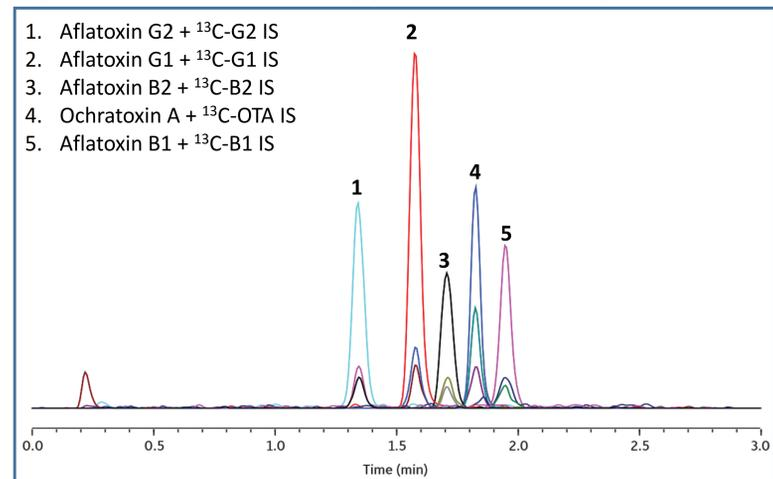
The method was applied to a commercially available CBD oil which resulted in the detection of Ochratoxin A with passing ion ratios, with the reported result below the LOQ. (Figure 5).
