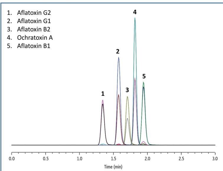
During column scouting, it was found that Raptor Biphenyl provided the best separation characteristics. The unique selectivity of the phase combined with the speed of superficially porous particles enabled the analysis to be performed in two minutes with a complete cycle time of only three minutes (Figure 2).
